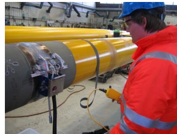
Inspection of new riser using Phased Array and Time of Flight Ultrasonic
